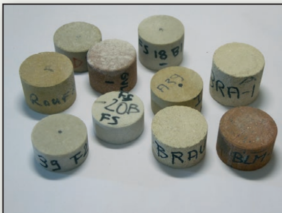
Plugs for porosity, air permeability, and formation factor.
