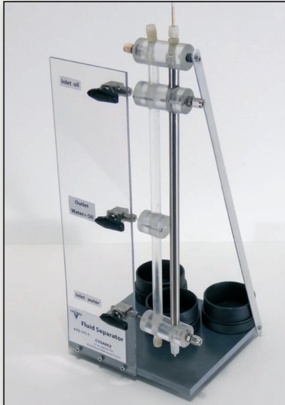
Separator with accurate level measurement by capacitance, with continuous recording.
