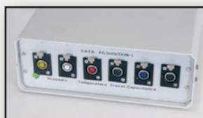
Data acquisition board, interfaced with software CYDAR.
