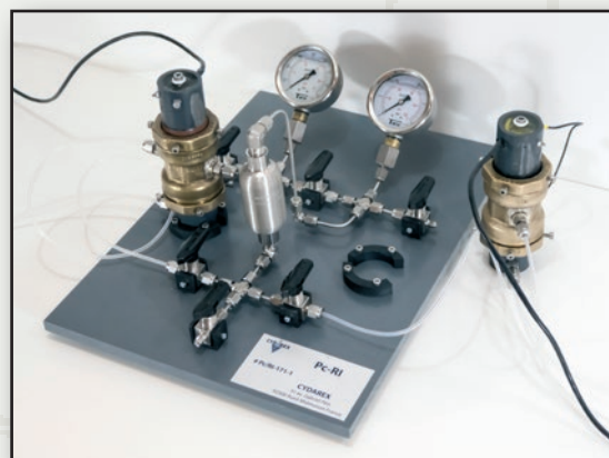
Pc/RI core holder and injection device.
