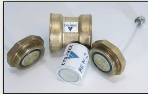
Core holder and plugs, with properties allowing fast measurements.
