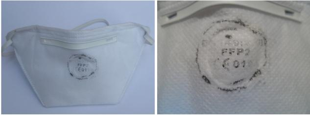
Figure 1: A FFP2 mask. India ink was used to assure that the permeability measurement was performed at the same location.
