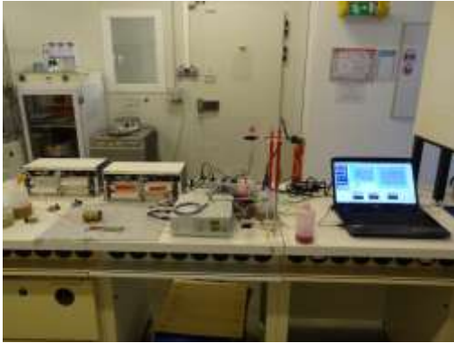
Figure 20: actual set-up. A double separator with a capacitance is used to record the variation of water level with time.
